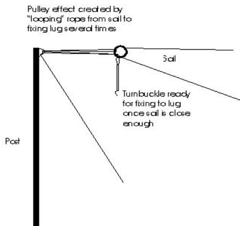
You may have access to purpose built pulley systems such as block and tackle, and if so we recommend you use them. Continue this process until all fixing points are in place. Your turnbuckles should still be fully unwound.
