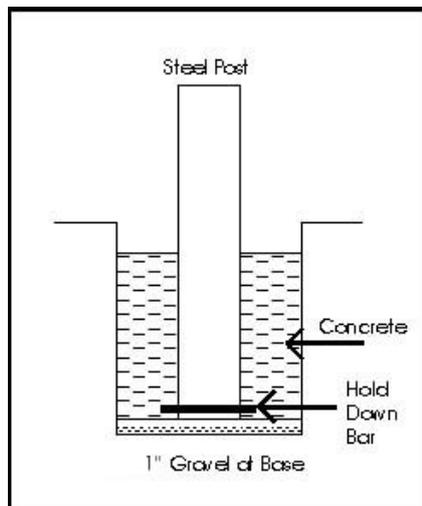
As a general rule, hole diameters should be around 350mm (1'2"), however increasing as column sizes increase. Depth, however, is the most important factor.
